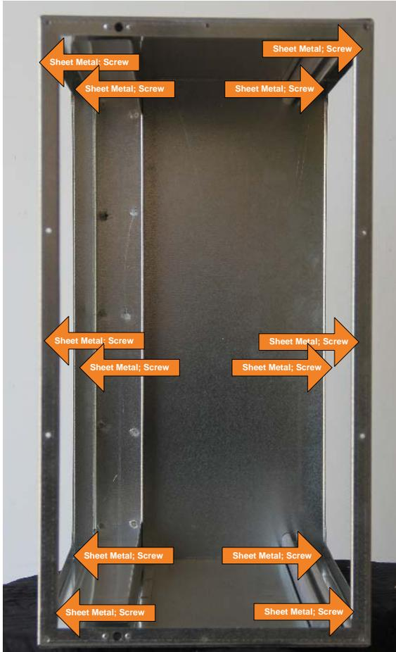
Image 5: Use sheet metal screws to fasten the CirrusAir chassis to existing duct and air handler from the inside
